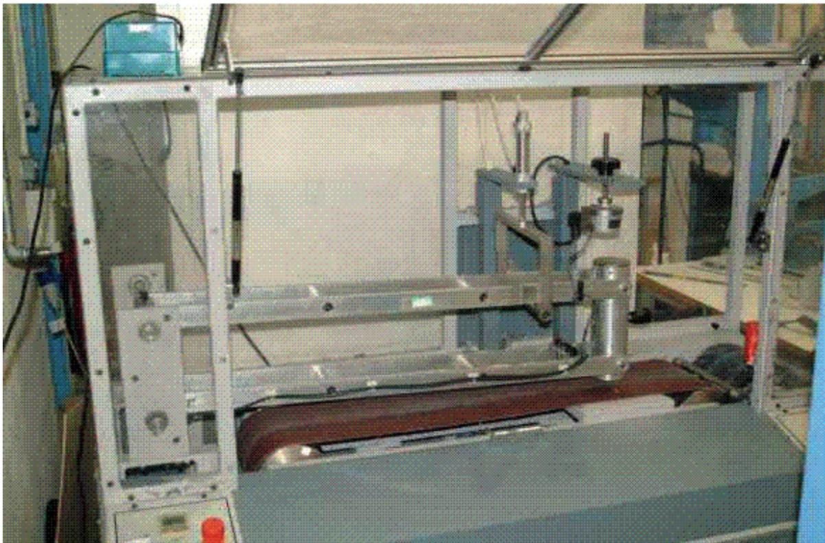
Picture 2: SATRA's EN 13595 "Cambridge-type" impact abrasion apparatus
